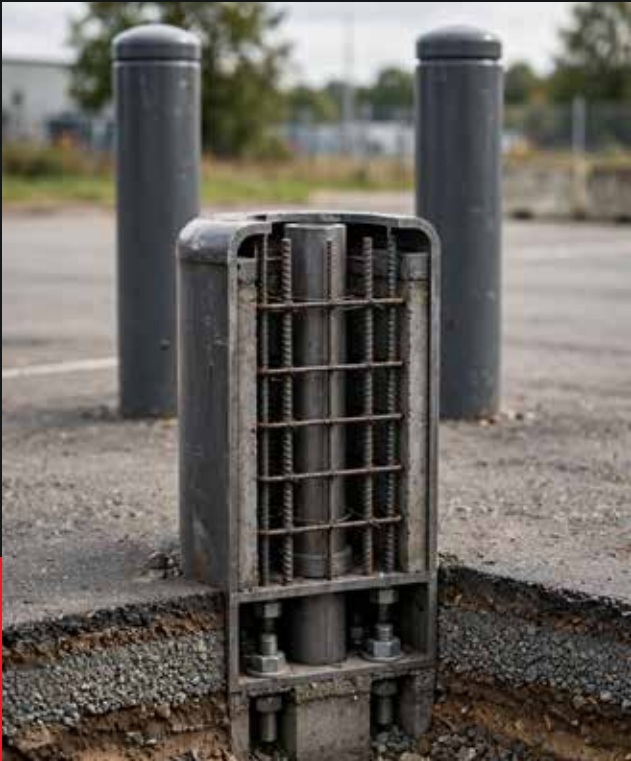
Reinforced Security Bollards
